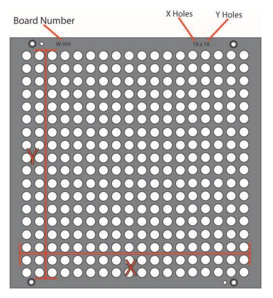
The holes per inch can be found at the top of the board (e.g. 7 x 9, 7 x 10).
